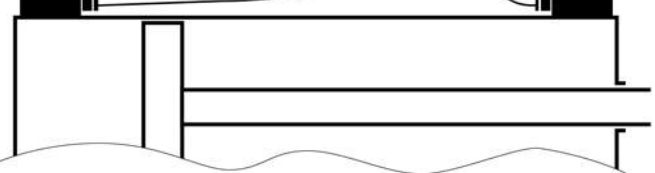
3 - Flow control fittings are fitted directly unto the cylinder ports if access is good.
