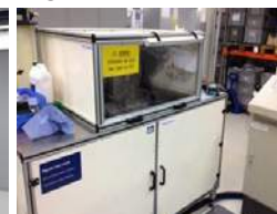
Impulse pressure test stand up to 4000 bar.
