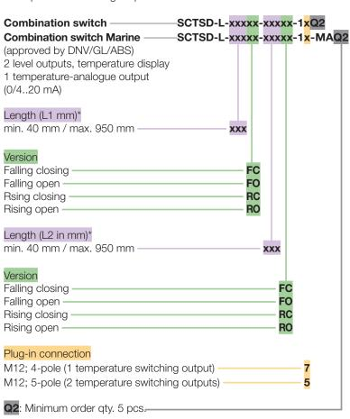
\*Switching output 1 (L1) can be above or below switching output 2 (L2) L1 and L2 are multiples of 10 mm Smallest difference between L1 and L2 = 30 mm
