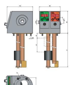
L1 = length of the sensor (mm) L2 = active range (mm)
