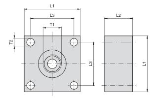
**SCAF-1/4-40** for mechanical pressure switch
