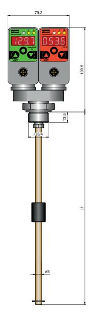
L1 = length of the sensor (mm) L2 = active range (mm)
